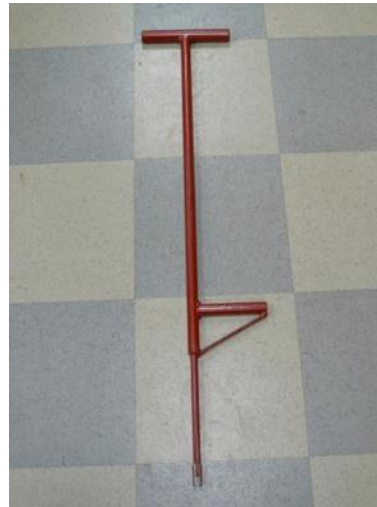
Tool for Installing “W” clips
